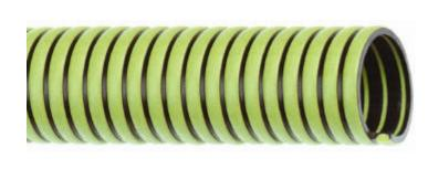
RN2 is a light weight and flexible rubber suction/discharge hose with a polyethylene helix designed for industrial and construction applications, as well as liquid waste, septic handling, agricultural applications and marine use. The external helix provides for easy drag, and it has a smooth bore. It is also a bit less expensive than some other rubber suction hoses. -40F to 158F.
